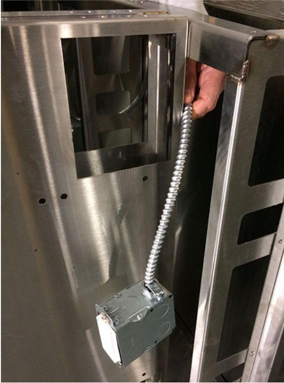
Line up and install 4 each #10 screws as shown here.
