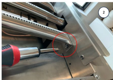
SAME THING FOR THE SCREW UNDER THE BURNER
