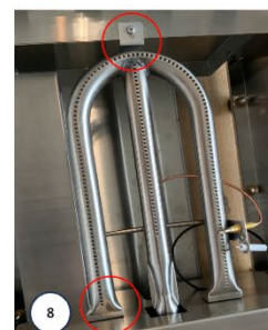
TIGHTEN THE SCREWS AT THE TOP AND BOTTOM OF THE BURNER
