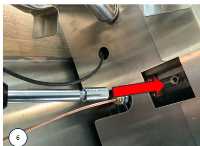
REINSTALL THE NEW ORIFICE FOR LP GAS (SIZE 0.9)
