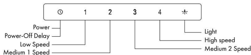
**Power:** Turn ON/OFF the range hood and activate power-off delay timer.
