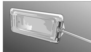
Hint: The screwdriver blade must be able to pass between the metal clips to reach the inner catch.
