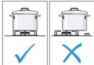
Position the cookware in the middle of the burner, otherwise it may tip over. Do not position large cookware on the burners close to the controls. The controls may be damaged due to overheating.
