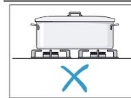
Never use multiple burners to heat up cookware, such as roaster, pan, grill stone. The build-up of heat that results from this will damage the appliance.
