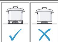
Place the cookware on the burner grates. Never place the cookware directly on the burner. Before using the appliance, ensure that the burner grates and the burner caps are positioned correctly.
