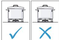
Do not use deformed cookware. Deformed cookware is not stable on the cooktop and may tip over. Use cookware with a thick, flat base.
