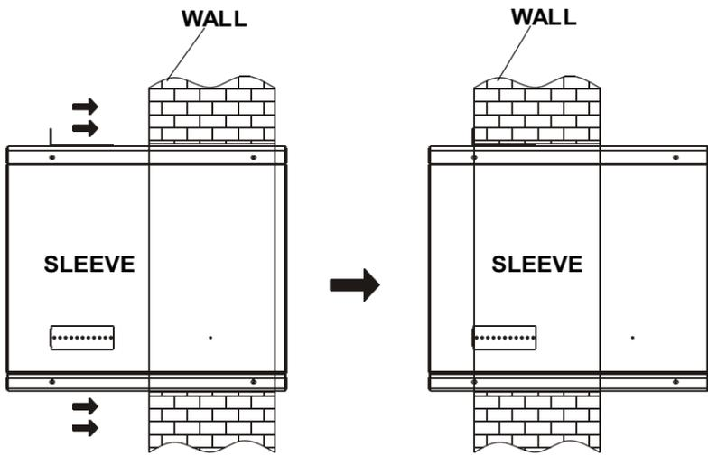
**INSTALL THE COVER PANELS(when not using air conditioner for a long time.)**
