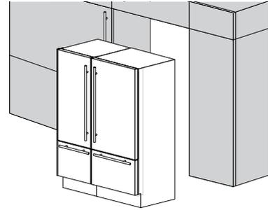
2. Access the back of the appliances to mount the joining brackets supplied in the Join Kit: Fix one side of the top and lower brackets to one of the appliances and subsequently to the other.
