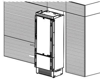
For a built-in installation, special side profiles are installed between refrigerator and adjacent cabinets.
