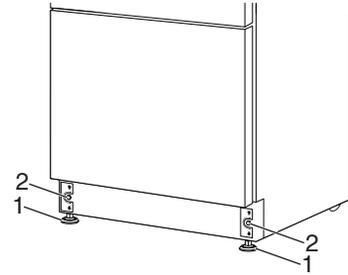
2. Adjust the leveling legs to level and align the refrigerator from left to right and front to back so that the refrigerator is level and aligned with the cabinets.
