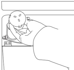
**IMPORTANT:** Air trapped in the water system may cause water and filter to eject. Always dispense water for at least 2 minutes before removing the filter or blue bypass cap.
