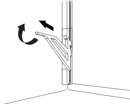
5. Place the support bracket at required height, slide in the support brackets on both sides. Make sure support brackets are placed at same height.
