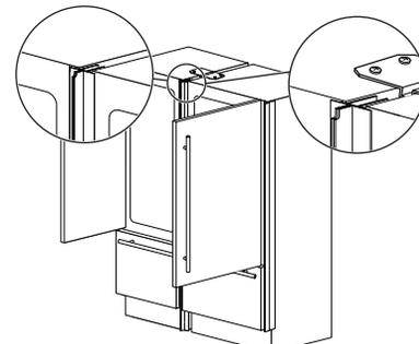
4. Finish off by mounting the center profile trim (C) onto the connected Profile Connection Trim (A) pieces by pushing it until a click is heard.
