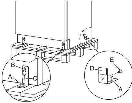
1. Unscrew the four bolts (A) by using 3/4" (19 mm) wrench.
