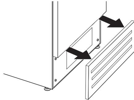
3. Use a vacuum cleaner with a soft brush to clean the grille, the open areas behind the grille, and the front surface area of the condenser.
