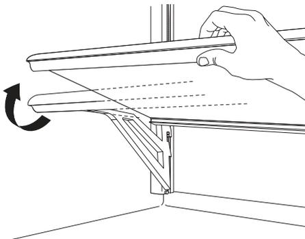
4. To adjust the glass shelves height, tilt the support bracket upward and pull out the bracket on both sides.
