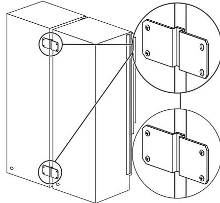
3. Next join them at the front by connecting the two Profile Connection Trim (A) pieces facing each other (x5) with the supplied screws. Attach the bracket on top of the units (if applicable) as per image.
