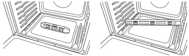
2. If range is not level, use a wrench or pliers to adjust leveling legs up or down until the range is level.
