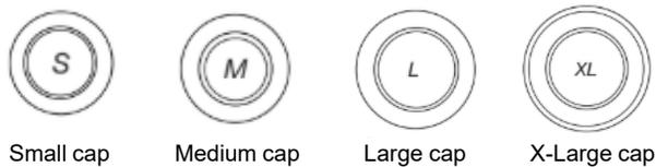
Burner caps should be level when properly positioned. If burner caps are not properly positioned, surface burners will not light. The burner cap should not rock or wobble when properly aligned.
