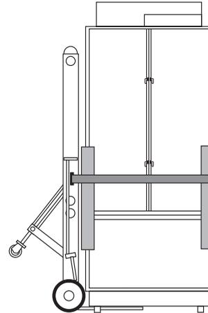
2. Place pieces of the shipping carton on the floor when rolling the dolly and refrigerator into the house. Move the refrigerator close to the built-in opening.
