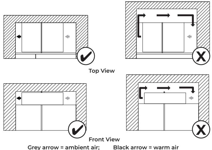
Cabinet depth 25" and soffit located at 84", provides proper airflow/ventilation to the refrigerator. Efficient cooling is achieved.
