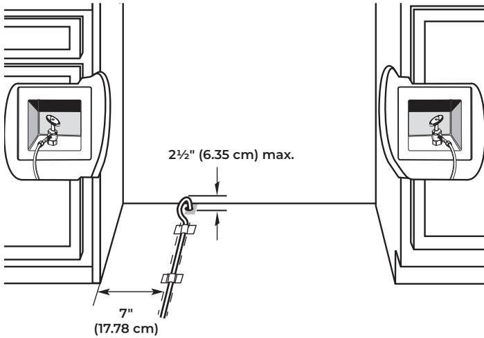
**NOTE :** The flexible, codes-approved water supply line should connect to the supply valve through the floor.
