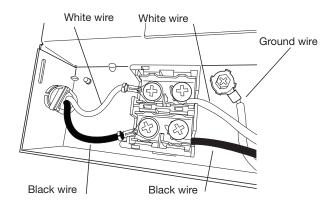
To connect wires with ring terminals, remove the screws from the terminal block, place the screw through the ring terminals, and reattach screws back into the terminal block.
