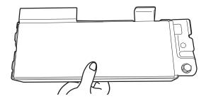
Place wires inside terminal box. Replace the cover by inserting the hooks of the terminal cover into the slots in the floor of the terminal box and sliding the cover tight against the back wall where wires come in. Make sure wires are tucked inside the box and not pinched by the cover. Put the terminal box back on the crossbar and push to the right so terminal box snaps into the plastic side member.
