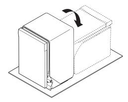
**Helpful Tip:** Remove all internal shipping material, drain hose, installation kit, and handle (if included,) before laying on it's back, and do not remove film on the door at this time.
