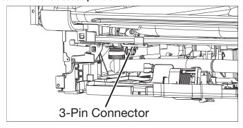
On some models, a service connection wire with a 3-pin connector is intentionally left unplugged and tucked behind the access panel. This is provided for use by the service technician.
