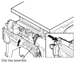
To remove the drip tray assembly, press the snap at each side of the plastic tray in toward the center of the product and pull toward yourself. Be sure not to pull too far or too hard as the float switch wire is still connected at this time.
