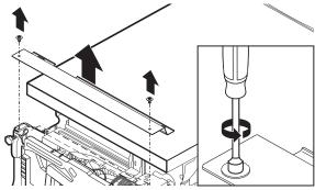
Using a 5/16" (7.9 mm) nut driver, remove the two screws attaching access panels to dishwasher. Once the screws are removed push the access panel toward the top of the product to unhook it and then remove it.
