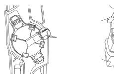
To remove the float switch wire, gently push the connector latch tab (1) and then pull the connector (2) out of the housing. The float itself should not be removed from the tray.
