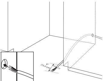
If installing with direct wire, route the cable as shown. Do not connect the wire to the product at this time. This connection will be made later, after the unit is installed into the cabinet opening.
