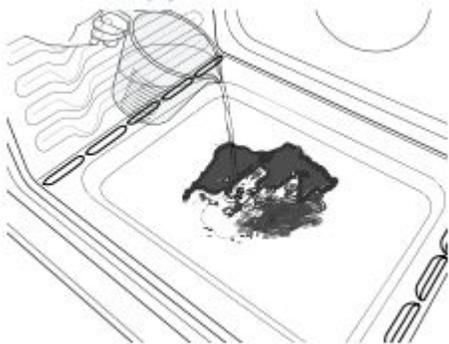
**IMPORTANT:** Do not use chemicals or other additives with the water. Do not open the oven door during the Clean cycle. The water on the oven bottom is hot.
