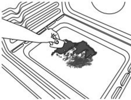
2. Pour 1<sup>3</sup>/<sub>4</sub> cups (14 oz [414 mL]) of distilled or filtered water onto the bottom of the empty oven, and close the oven door.
