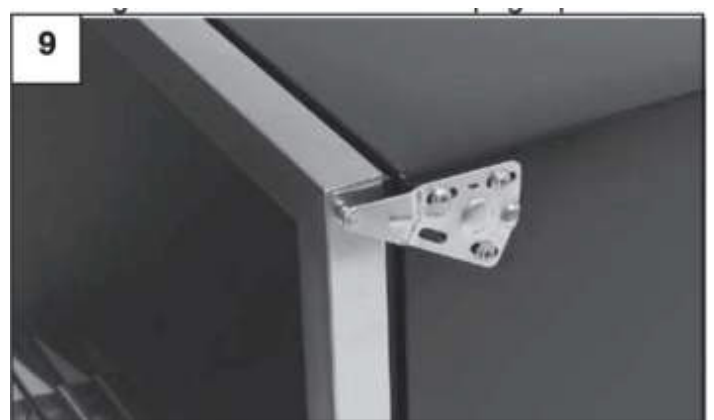
9. The rubber gasket should be compressed on all sides of the door. If the gasket is more compressed on one side, the metal bracket position should be adjusted. Make sure the door is level. Once the door position is finalized, securely tighten the screws.
