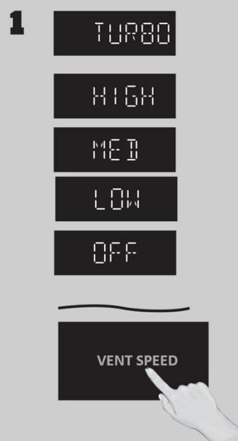
The Fan (Vent Fan) removes steam and other vapors from the cooking surface below the microwave oven. Press **Vent** Fan pad once for **Turbo** fan speed, twice for **High** fan speed, 3 times for **Med.** fan speed, and 4 times for **Low** fan speed, 5 times for fan speed off.
