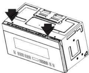
Remove 2 grille screws to remove the grille.
