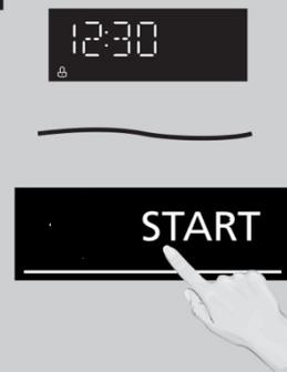
When the time of day appears in the display, press **Start** three times; Current time will appear in the display.
