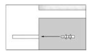
Fit the brackets (item No.1) into their places, using 4 screws for each. You must use all of the 2 brackets to ensure safety of the product.
