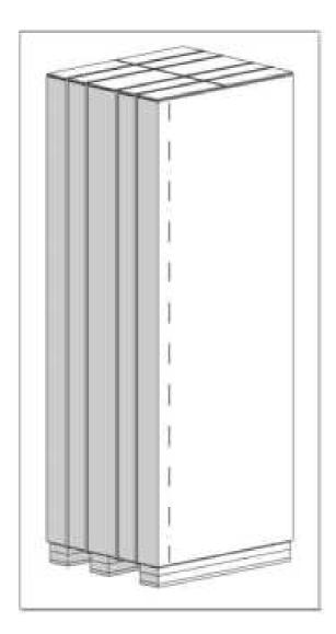
Remove the Packaging Polystyrene material.
