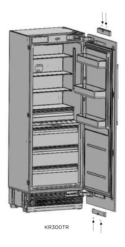
After the top and bottom door panel brackets are secured by installing screws,
