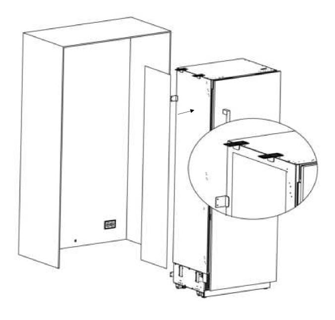
Bring the two refrigerators side by side. After making sure that they are in alignment, screw the fasteners (4) to the other refrigerator.
