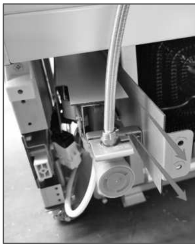
2. Pull out the water valve fixing bracket outward
