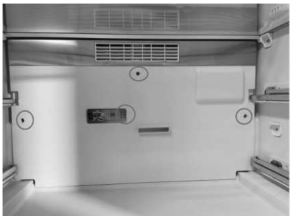
1. Remove the cover plate fixing screws
