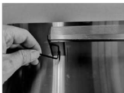
1. Use an Allen wrench to remove the set screw on the side of the handle base
