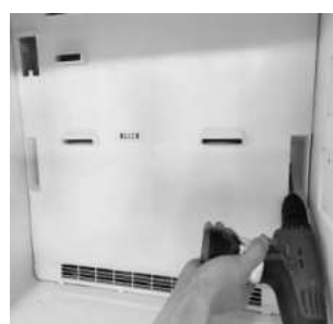
2. Remove the air duct fixing screws
