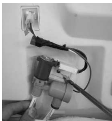
1. Remove the fixing screws and water pipes
