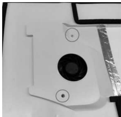
4. Remove the fan cover fixing screws
