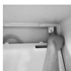
4. Unplug the terminal block and remove the cover plate
