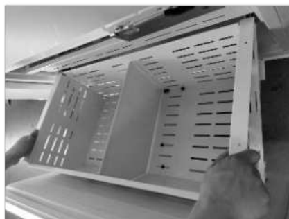
1. Pull out the freezer door body and remove the 4 handscrews
