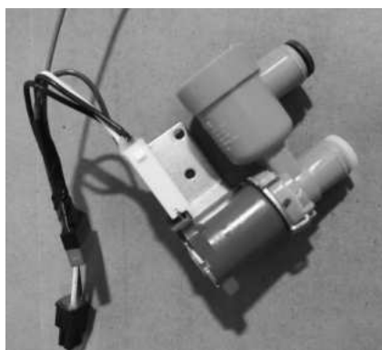
2. Unplug the terminal to remove the watervalue
