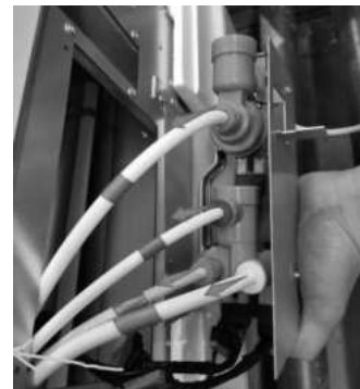
3. Pull out the water pipes on the water valve one by one
