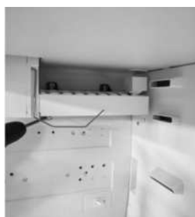
3. Remove the screws holding the ice maker in place
