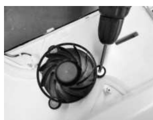
7. Removing the freezing fan
