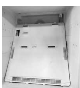
3. Remove the air duct cover
