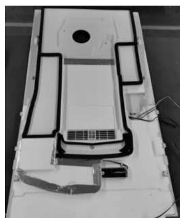
3. Remove the air duct coverplate
