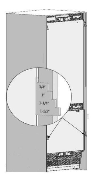
Position of the level adjustment part (10) must be adjusted according to the thickness of the door. It can adjust the level for 4 different door thickness levels.
