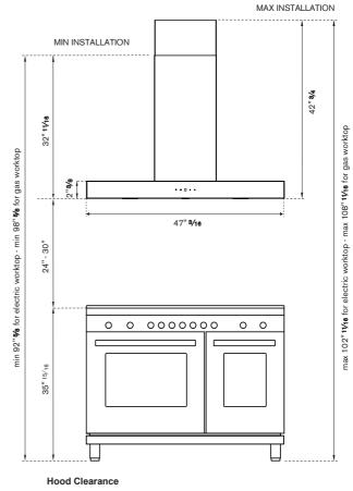
Recommended height above cooking surface: min 24" for electric worktop min 30" for gas worktop
