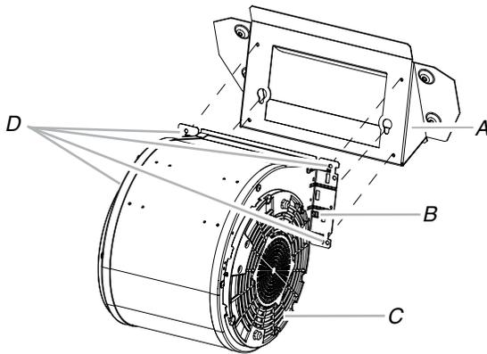
A. Rear motor mounting bracket    C. Blower motor
