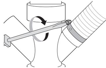
**Connecting to Disposal or Waste Tee with Air Gap**
