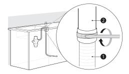
If it is not connected, attach the rubber hose connector to the disposal or waste tee with a hose clamp (not provided).
