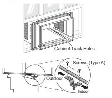
**5** Install the cabinet with a slight tilt (about 1/2") downward on the outside.
