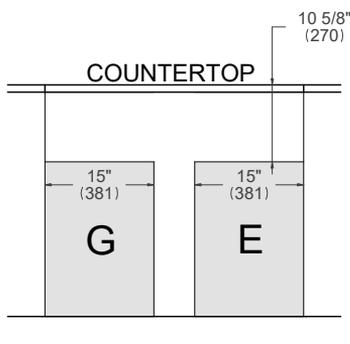
**E** A properly-grounded, horizontally-mounted electrical receptacle should be installed according to this drawing.
