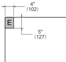
For single ovens installed into a wall cabinet, the electrical junction box may be located above, below to the left or right of the unit within reach of the power cord. Placement within the opening may require additional cabinet depth.
