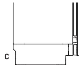
\* If a shaker style panel is used, which is thinner than the minimum panel thickness, shorter screws than those supplied in the accessory pack must be used.
