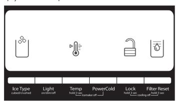
For your convenience, your refrigerator and freezer temperature controls are set to the recommended set points at the factory. When you first install your refrigerator, make sure the temperature controls are still set to the recommended set points. The recommended set points are 37°F (3°C) for the refrigerator and 0°F (-18°C) for the freezer.
