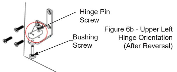
5. Using a 5/32" Hex Key, remove the Upper and Lower Hinge Brackets from the door (Fig. 7), saving all components. Remove black plugs from opposite side of door. flip the Upper Hinge Bracket and reattach the Hinge Bushing (Fig. 7) and screw into place on the opposite side of the door (where plugs were removed). Remove the Cam Closer from the Lower Hinge Bracket (Fig. 7) and attach it to the opposite side (Fig. 7b).
