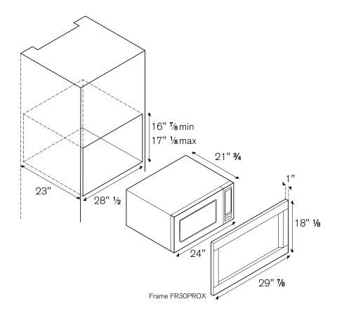
The minimum gap between the kichen cabinet upper or lower panel and the appliance is 1/8. This dimension must be added to the height listed in the drawings
