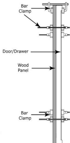
4. Secure integrated panel to door using clamps. A robust tape may also be used. Marvel recommends the use of bar clamps to secure the panel to the door. If using tape, be certain the tape will not damage panel finish upon removal.
