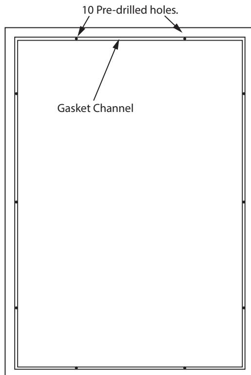
6. Using a  $\frac{7}{64}$ " drill bit, drill 10 pilot holes into the wood panel  $\frac{1}{2}$ " deep using the holes in the door frame as a guide.
