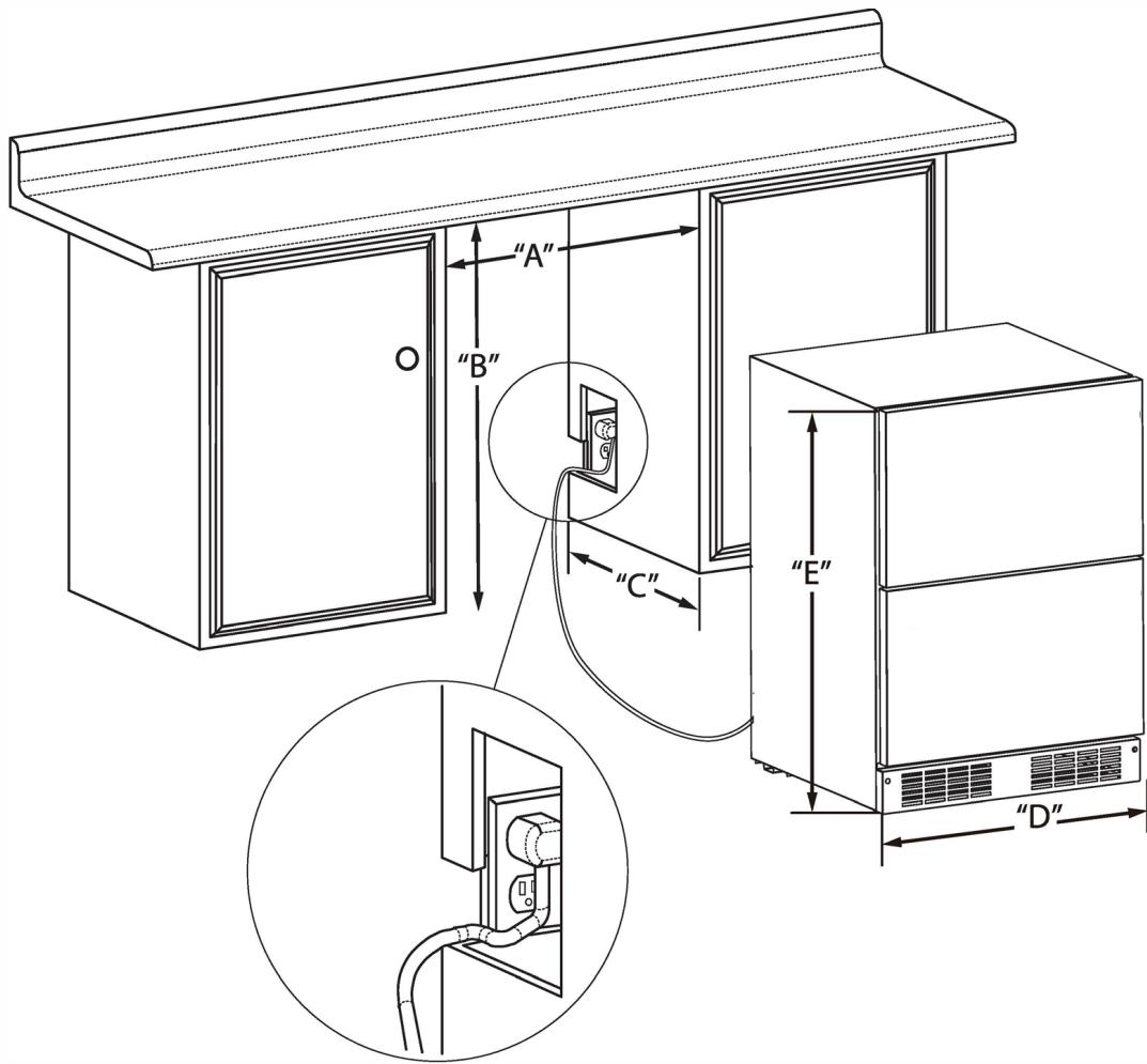
If necessary, to gain clearance inside the rough-in opening, a hole can be cut through the adjacent cabinet and the power cord routed through this hole to a power outlet. Another way to increase the available opening depth is to recess the power outlet into the rear wall to gain the thickness of the power cord plug. Not all recessed outlet boxes will work for this application as they are too narrow, but a recessed outlet box equivalent to Arlington #DVFR1W is recommended for this application.
