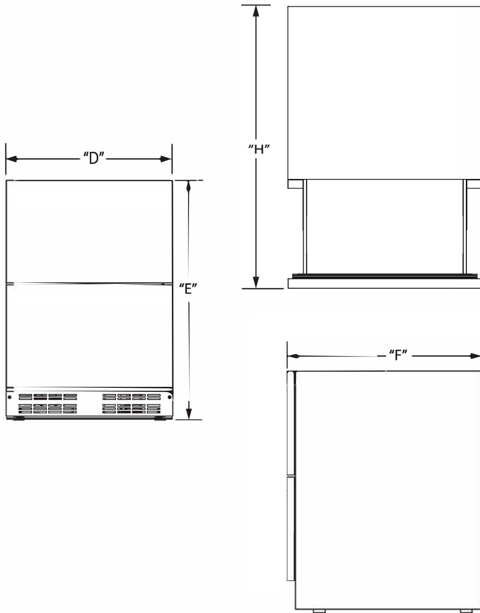
Minimum rough-in opening is required to be larger than the adjusted height of the cabinet.
