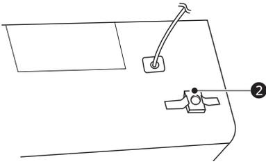
**3** Cut or drill a 2" diameter hole at the area marked "M power supply cord hole" on the upper cabinet template. If the upper cabinet is metal, you will need to cover the edge of the hole with the power supply cord bushing (supplied) to prevent damage to the cord from the rough metal edge.
