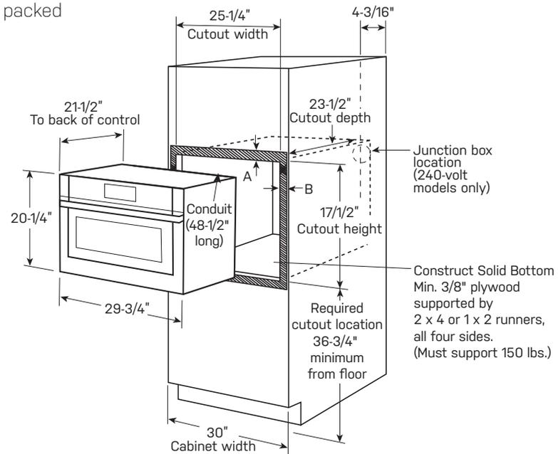
A / B = Allow the following clearances around the cutout on the front surface of the cabinet: 1-7/8" from the top, 2-3/8" from the side edges and 1-1/8" from the bottom.
