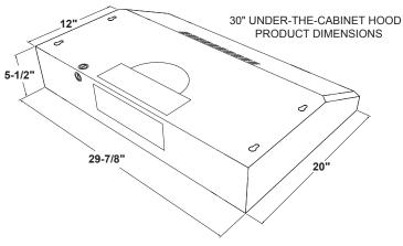
Exhaust outlet connects to  $3\text{-}1/4" \times 10"$  rectangular duct. Vent top or rear. Includes rectangular damper.
