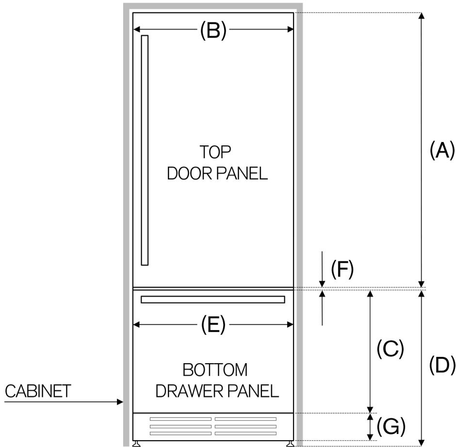
**NOTE:** These specifications assume a standard toe kick height of 4". For different toe kick heights, adjust C accordingly.
