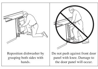
**4** Push dishwasher completely into the opening so that the front corners of the dishwasher door are flush with the cabinet doors.
