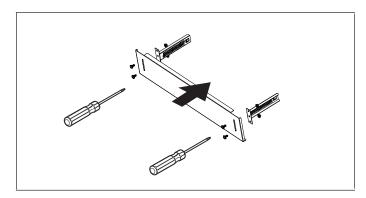
**5** Insert the bracket into the corresponding hole on the dishwasher chassis. If you still need to adjust the height position, please remove it and reassemble it.
