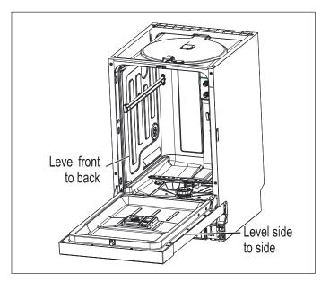
**NOTE:** Pull lower rack out about halfway. If the rack rolls forward or back into the dishwasher, the dishwasher must be leveled again.
