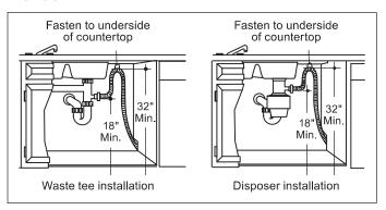
**IMPORTANT:** When connecting drain line to disposer, make sure that the drain plug has been removed. DISHWASHER WILL NOT DRAIN IF PLUG IS LEFT IN PLACE.
