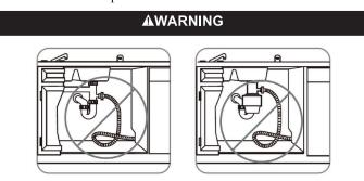
Do not connect the drain hose to the sink drain waste tee or garbage disposal without looping the drain hose underneath the sink with a high drain loop. Doing so will cause the dishwasher to not drain properly, which may allow drain water to back up in the dishwasher tub or result in an E1 error code.
