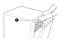
Align the dishwasher with the opening. Make sure the water supply line and electrical cable are in the correct positions to slide into their channels properly.
