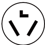
3-Wire receptacle (10-30R)
