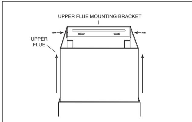
14 Slide the upper flue upward until it is aligned with its upper flue mounting bracket. The bracket should be inside the flue. Secure the upper flue to the upper flue mounting bracket using (2) no. 8 x  $\frac{3}{8}$ " mounting screws.
