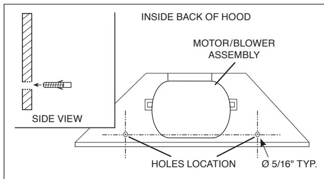
11 With the hood hanging in place, drill through both holes located in the inside lower back of hood using a  $\frac{5}{16}$ " drill bit. Insert the included drywall anchors into the drilled holes (one for each hole). Install (2) washers and (2) no. 8 x  $\frac{1}{2}$ " mounting screws through the hood back and into the drywall anchors. Verify that the hood is centered and leveled. Tighten all screws completely.
