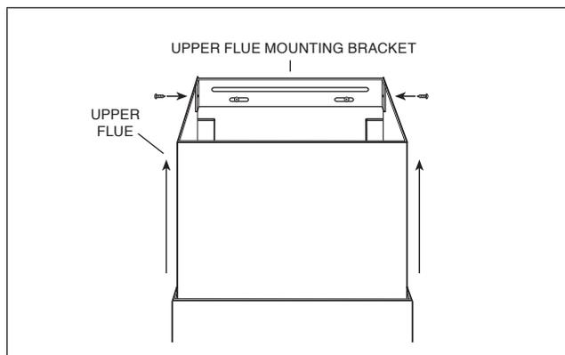
13 Slide the upper flue upward until it is aligned with its upper flue mounting bracket. The bracket should be inside the flue. Secure the upper flue to the upper flue mounting bracket using (2) no. 8 x 3/8" mounting screws.
