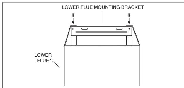
NOTE: 10-ft. ceilings require 10-ft. Flue Extension Model SKCH62EXF (sold separately). Discard the upper flue supplied with your hood and replace it with the Model SKCH62EXF flue extension.
