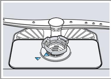
3. Check the outlet nozzles on the spray arms for blockages under running water and remove any foreign objects.
