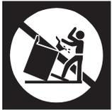
**⚠WARNING** To reduce the risk of tipping of this appliance from abnormal usage by excessive loading of the Microwave Drawer™ Oven, the appliance must be secured by installing the Anti-Tip device supplied. If it is not, there is a risk of the product tipping and causing injury if someone stands, sits or leans on the open drawer. Please refer to the Anti-Tip device information in the Installation Manual.
