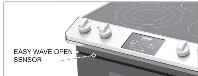
To use the Easy Wave Open feature, simply wave your hand in front of the sensor in two consecutive motions, either up and down or side to side.
