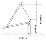
The free end should be positioned at a height of between 30 and 100 cm (11" 13/16 and 3' 3" 3/8) , and should never be submerged in water.
