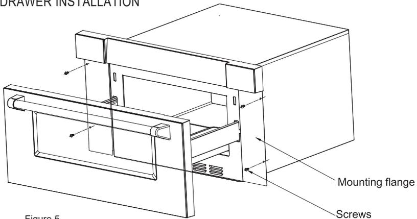
1. Place the drawer adjacent to the wall or cabinet opening. Plug the power supply cord into the electrical outlet.
