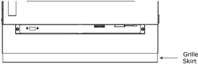
1. Loosen, but do not remove, the lock screws on the inside of the grille rails. Lock screws are located on the inside of each grille rail.
