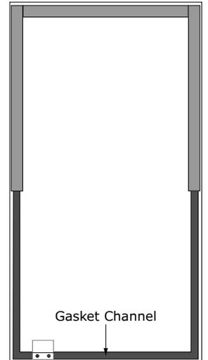
5. Install plunger bracket at the opposite corner, utilizing the 2 pre-drilled holes.
