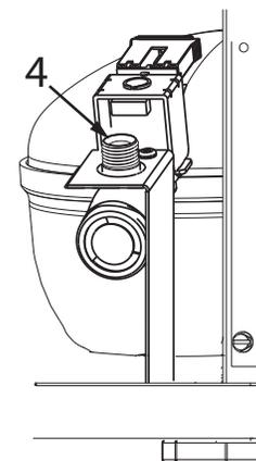
5. Turn on water supply and check for leaks.
