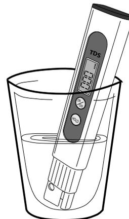
5. Leave meter immersed for 30 seconds.
