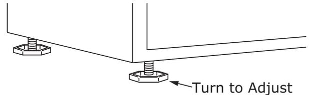
3. Confirm the unit is level after each adjustment and repeat the previous steps as needed.
