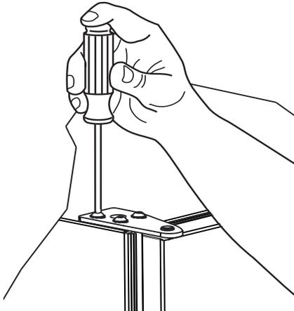
4. Tighten three screws and replace hinge cover.
