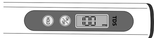
7. Turn off meter, dry off, and replace cap.
