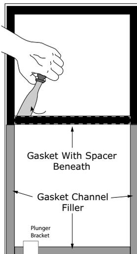
4. Take out 2 screws and remove plunger bracket from gasket channel.
