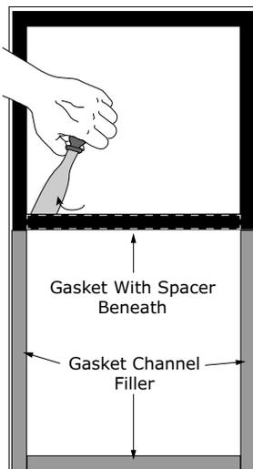
4. Install gasket into channel, beginning at one corner and pressing in firmly.
