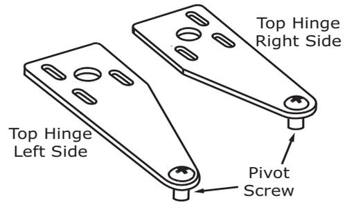
1. Remove pivot screw from hinge, flip hinge over, and install the pivot screw in the same hole from the opposite surface.
