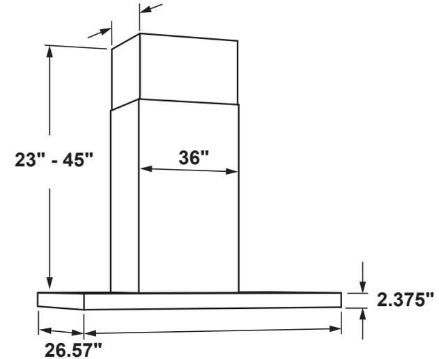
The vent hood must be installed 24" min. above the cooking surface. For optimal performance, installing the hood more than 38" above the cooking surface is not recommended. The hood installation height above the cooking surface depends upon the ceiling height. The telescopic duct cover conceals the ductwork running from the top of the hood to the ceiling.
