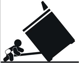
A child or adult can tip the range and be killed. Check installation of anti-tip device per installation instructions.
