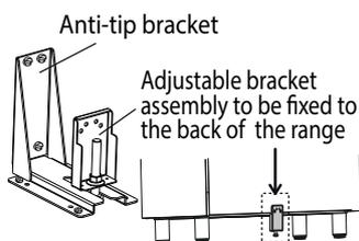
To verify the anti-tip bracket is installed and engaged:
