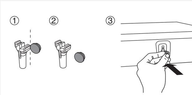
**3** Remove the caps from the plastic plugs. Push the caps over the three holes in which the plastic plugs were inserted. Save the bolts and plastic plugs if you have to transport your washing machine in the future.
