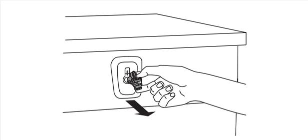
**2** To remove the plastic plugs holding the bolts, squeeze them and then pull them out.
