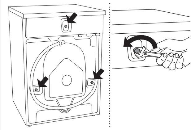
**1** Release and remove the bolts as shown in the figures.
