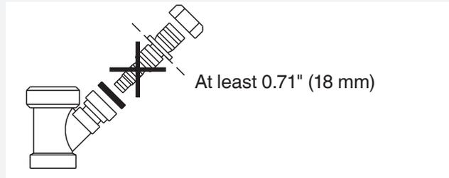
💡 If the hose is extended, the internal diameter of the coupling must not be less than 1/2" (12.2 mm).
