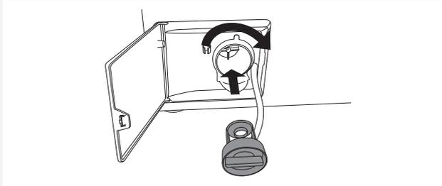
**6** Replace the filter as shown in the figure and fasten it by rotating in the clockwise direction. For a good seal, the filter seal surface should be clean. Also re-install the drain hose.
