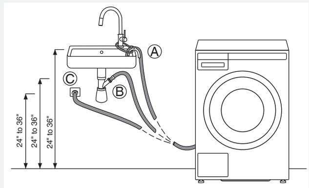
Drain hose can also be connected directly to the washbasin drain via a siphon. In this case, the hose, too, should be 24" to 36" (610 mm to 914 mm) above the floor. Internal hose diameter should be at least 0.71" (18 mm). See figure.
