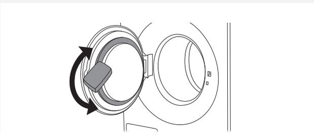
**1** Press the tab to completely remove the detergent compartment from its housing.
