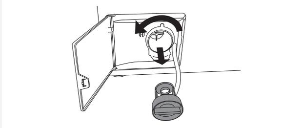
**3** Gradually rotate the filter in the counter-clockwise direction and pull it out.
