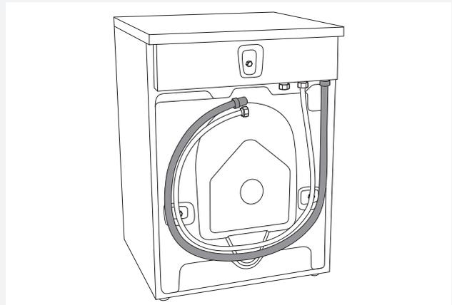
The machine is supplied with the outlet hose already attached. The hose should be extended over a suitable sink edge or drain pipe at a height of 24" to 36" (610 mm to 914 mm) above the bottom of the unit. (The lower height is preferable.) Make sure the hose is not kinked.
