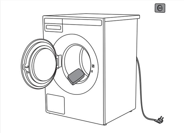
Connect the washing machine to the power mains and run the dedicated drum cleaning program. See chapter "WASHING PROCESS" /STEP 5: CHOOSE THE PROGRAM.
