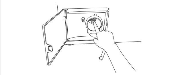
**5** Remove all objects and impurities from the filter housing and the impeller.
