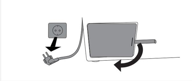
**1** Before cleaning, drain the water from the washing machine using the Drain program, and disconnect the washing machine from the power mains.
