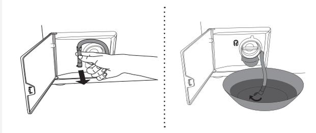
**2** Release the water drain hose from the holder.
