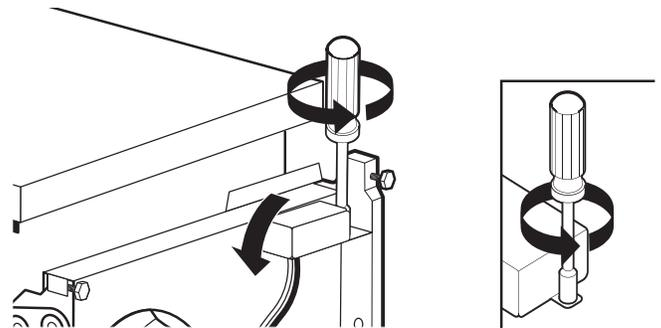
Using a 1/4" hex-head socket, nut driver, or Torx® T20® screwdriver, remove terminal box cover. Retain for later use.
