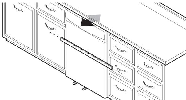
Align front of dishwasher door panel with front of cabinet doors. You may need to adjust alignment to be even with your cabinets.
