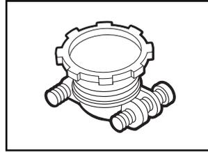
**Household Wiring (Metallic) Strain Relief to fit 7/8" (22 mm) hole** (required to properly secure household wiring to the dishwasher terminal box)
