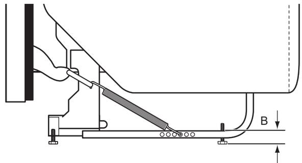
Adjust both front and back leveling legs to the same height.
