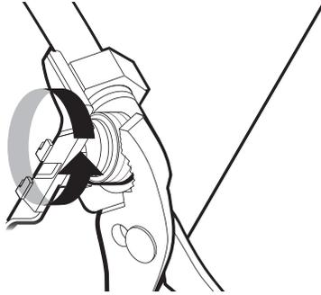
Be sure rubber washer is properly seated in fitting. Slide the 3/4" (19 mm) fitting of the 90° elbow up to the valve and hand-tighten to avoid cross-threading. Hand-tighten until the coupling is tight. Using pliers, check the tightness of the coupling. An additional 1/4 to 1/2 turn may be required to seal the rubber gasket. Route fill hose out the rear left side of unit.
