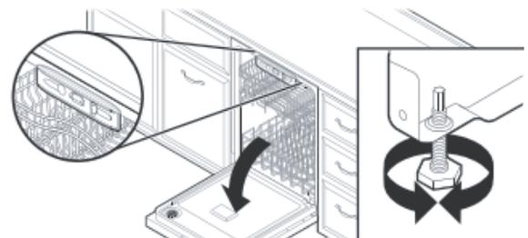
Place level against top-front opening of tub. Check that dishwasher is level from side to side. If dishwasher is not level, adjust front legs up or down until dishwasher is level.
