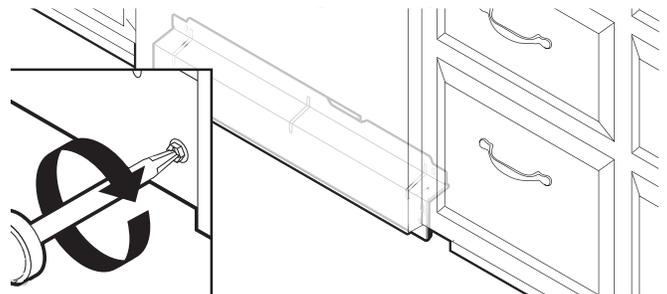
Tighten access panel screws.
