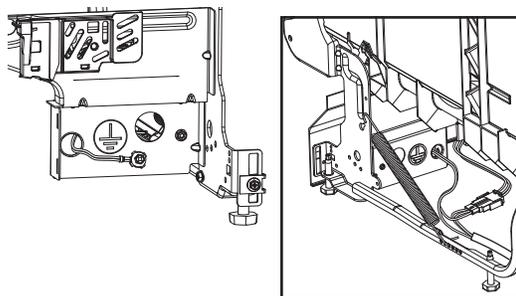
Select products include a factory installed power cord. For these products, no wiring during install is required. A ground wire to chassis connection is made inside the existing terminal box, and the normal terminal box cover is not included.
