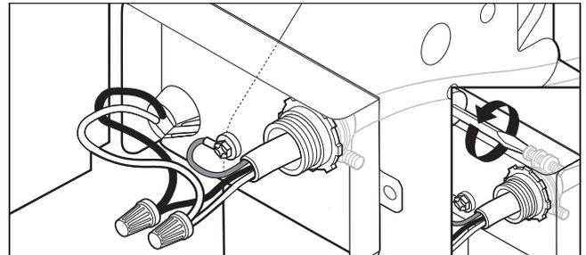
Tighten strain relief screws to secure cable.
