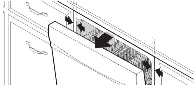
Open door and check that space between dishwasher cabinet opening and tub is equal on both sides. If spacing is not equal, loosen bracket screws and shift tub. Tighten bracket screws.
