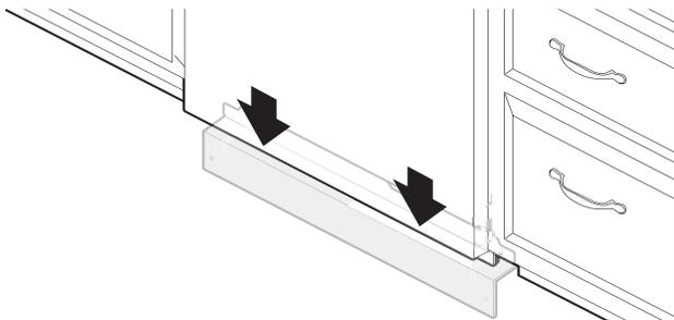
Check that the lower edge of the access panel touches the floor. Adjust if necessary.
