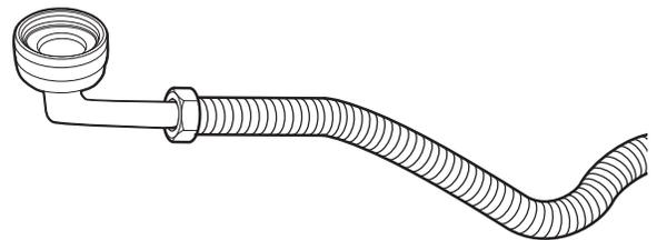
Get 3/8" (9.5 mm) compression x 3/4" (19 mm) hose fitting with 90° elbow. See the “Tools and Parts” section at the front of the guide for part details and order. Connect the 3/8" (9.5 mm) compression fitting of the 90° elbow fitting to the water supply line. Attach so the 3/4" (19 mm) connection is facing upward as shown above.
