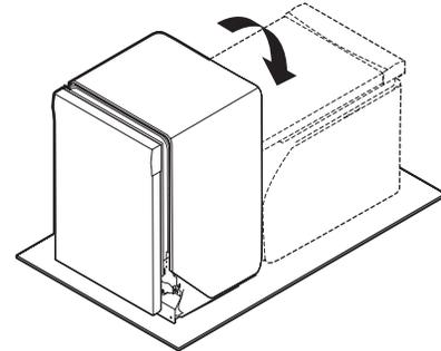
**Helpful Tip:** Place cardboard under dishwasher until installed in cabinet opening to avoid damaging floor covering.
