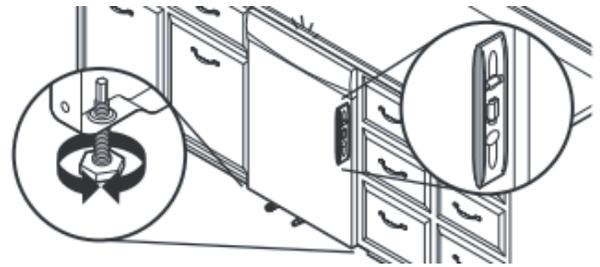
Check that leveling legs are firmly against the floor. Close and latch the door and place level against the front panel. Check that dishwasher is centered from front to back in the opening. If needed, adjust leveling leg until dishwasher is plumb. Repeat for other side of dishwasher.
