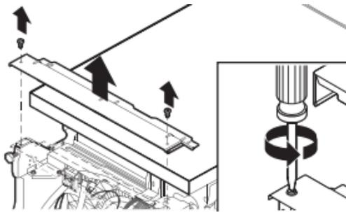
Using a 1/4" (6.35 mm) nut driver or Phillips screwdriver, remove 2 screws attaching access panel to dishwasher.
