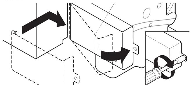
Place wires inside terminal box. Insert tabs on left side of cover. Make sure wires are tucked inside box. Close cover ensuring wires are not pinched. Use 1/4" nut driver or Torx® T20® screwdriver and previously removed screw to secure cover.
