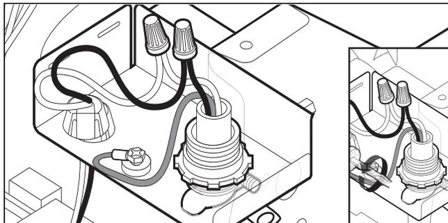
Tighten strain relief screws to secure cord.
