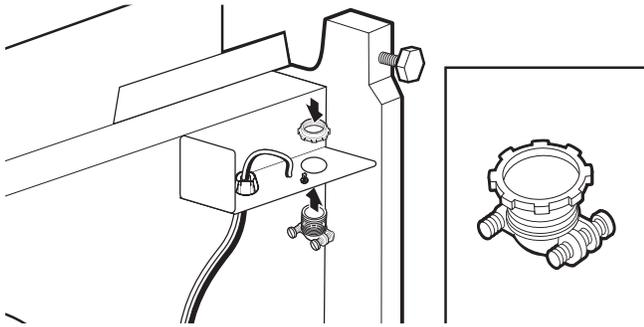
Install the metallic strain relief provided in this kit (Straight: Whirlpool Part Number 4317824, 90°: Whirlpool Part Number W10278923RP). Make sure screw heads are facing to the left when tightening conduit nut. Strain relief is provided with the power cord kit.
