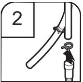
2. Attach drain hose to air gap with large drain hose clamp (provided). Use pliers to squeeze clamp open and move into position. If the drain hose was cut, use a 1 1/2" to 2" (38 mm to 50 mm) screw-type clamp (not provided).
