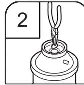
2. Use needle-nose pliers to remove plug.
