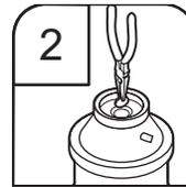
2. Use needle-nose pliers to remove plug.
