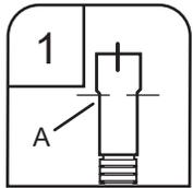
1. Fit rubber end (A) of drain hose to waste tee and cut if needed.
