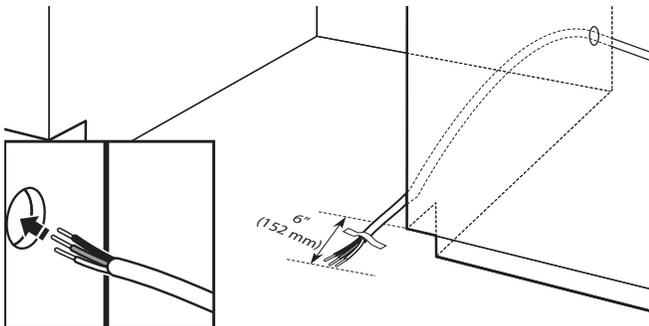
If installing with direct wire, route the cable as shown.
