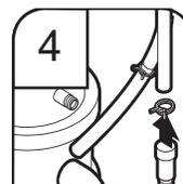
4. Attach drain hose to air gap with large drain hose clamp (provided). Use pliers to squeeze clamp open and move into position. If the drain hose was cut, use a 1 1/2" to 2" (38 mm to 50 mm) screw-type clamp (not provided).
