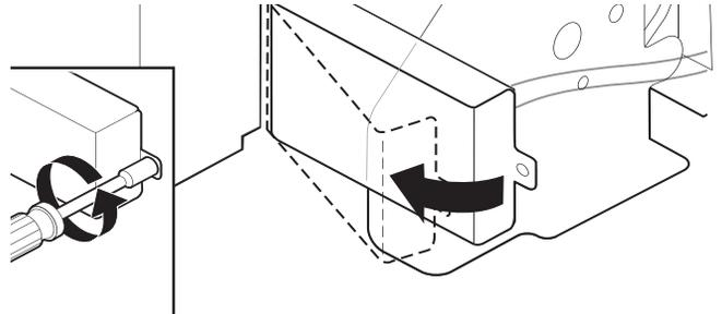
Using a 1/4" hex-head socket, nut driver, or Torx® T20® screwdriver, remove terminal box cover. Retain for later use.
