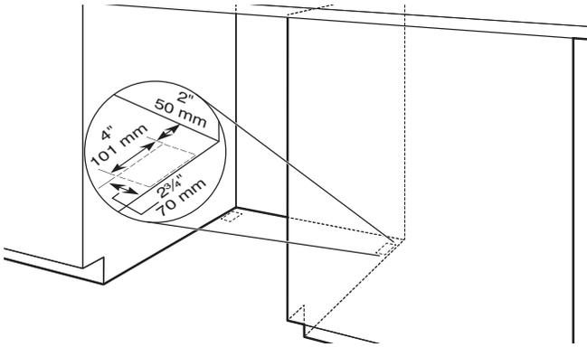
Built-up floors: If the kitchen floor is higher than the cabinet opening's floor—for example, the kitchen floor tile does not extend into the cabinet opening—add shims, as needed, in the area shown to bring the dishwasher up to 34" (864 mm) below the countertop.
