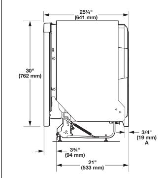
A. Insulation may be compressed (not used on all models).
